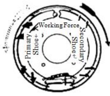
Fig 5-4 Brake Actions during Reversing Process
