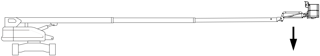
Fig 2 Position of lowest forward stability of the machine
