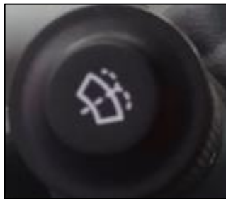
Fig.3.2.9 Front windshield spray switch
