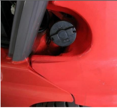
Fuel reservoir cap without lock
